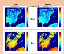
VIIRS and SEVIRI LST(°C) collocated in space & time, averaged over 1-9 Jan 2014: VIIRS night-time (top) and daytime (bottom) overpass
