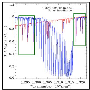
Fractional depth of absorption features decreases with an additive signal (e.g. SIF)
